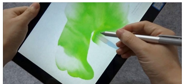
Figure 2: Tilting device to direct ink flow using G-Sensor.
